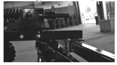
to torque specs (Page45). Raise roller basket assembly with hoist to reinsert top pin.
