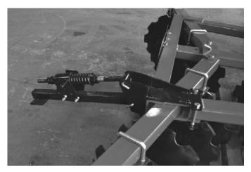
this step. Failure to do so will not allow the bracket to mount properly. Next attach the arm and spring rod assembly using the two mount pins (Photo 32). After both sides have been mounted start assembling the roller baskets together (if two baskets are used). Outer hangers are pre assembled onto the
