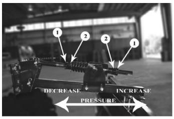
hex nut to create a lock. Tighten the forward facing hex nut on the front of each spring rod assembly to apply pressure on the spring (Photo 39). Once desired pressure is applied tighten the jam nut to create the lock. Make
