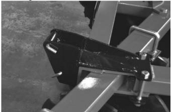
end of the frame angle iron. (Photo 31). Tighten the front and rear bolts evenly during
